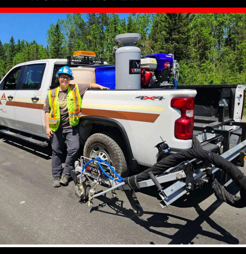
Pickup Truck-Mounted Road Marking Kits
