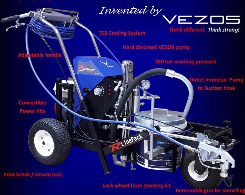
Runner LinePack accessory, transform the unit from a texture / paint airless sprayer instantly into a line striping machine. No tools needed in order to set up, simply roll the airless towards the kit and all will click into place, attach the steering kit on the main handle and start striping!
